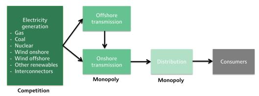
balancing the supply of electricity with the demand. This physical supply chain is illustrated in Figure 9.6.
